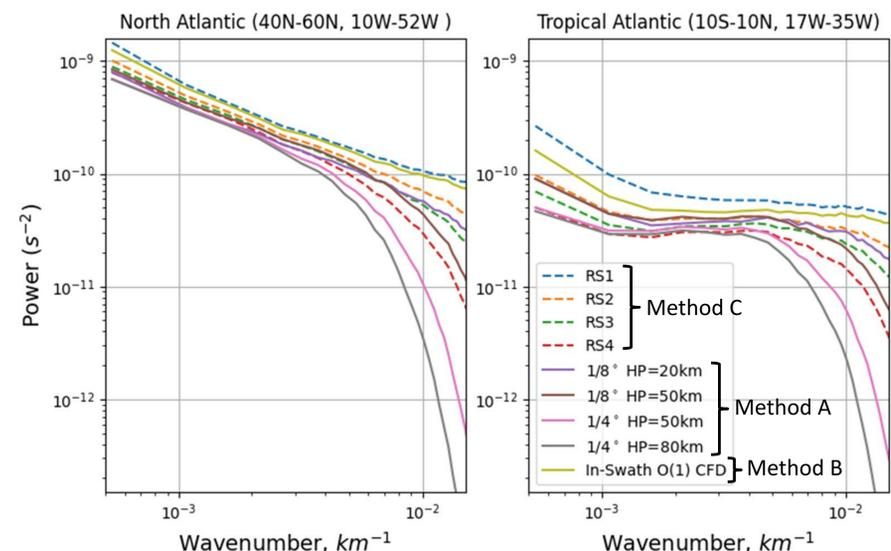
**Figure 3.** Spectra comparisons of vorticity for January 2008. RS1-RS4 are the ring sizes used with method C (see Fig. 1). The grid size and loess half-power filter cutoff limit are given for method A.
