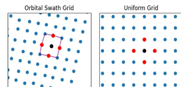
**Figure 1.** Left: Orbital swath grid used for methods B and C. Right: Uniform grid used for method A. Red dots indicate points used for centered finite differences. For method C, the purple line connects the points used in the line integral approach. With the 12.5km QuikSCAT data, this has a "ring size" of 25 km across (ring size 2).
