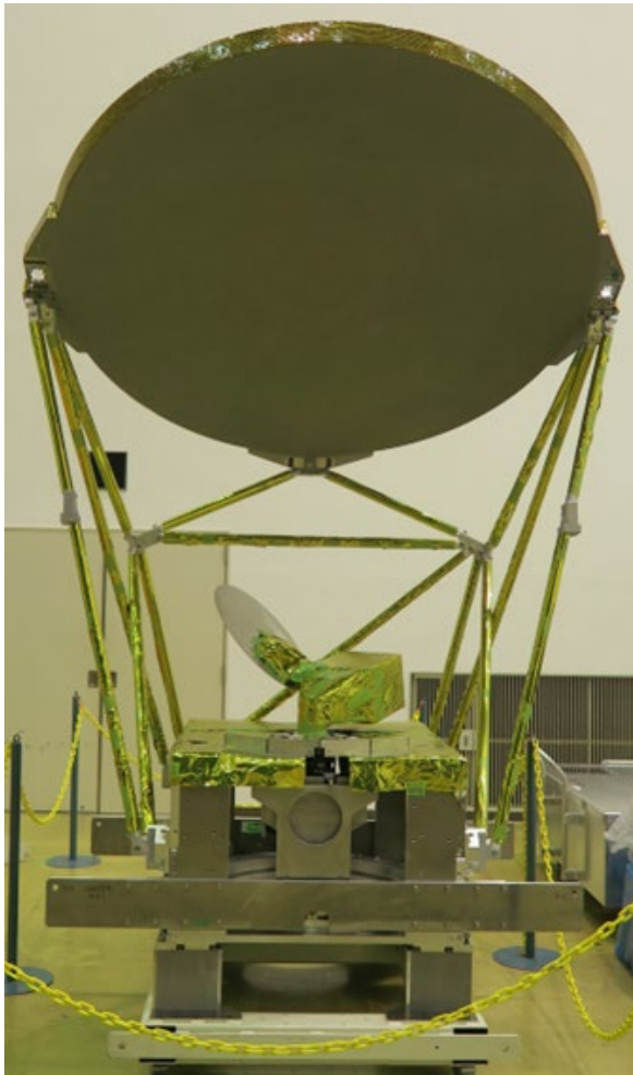
AMSR3 sensor in production. Photo: AMSR3 Main Reflector at Tsukuba Space Center
