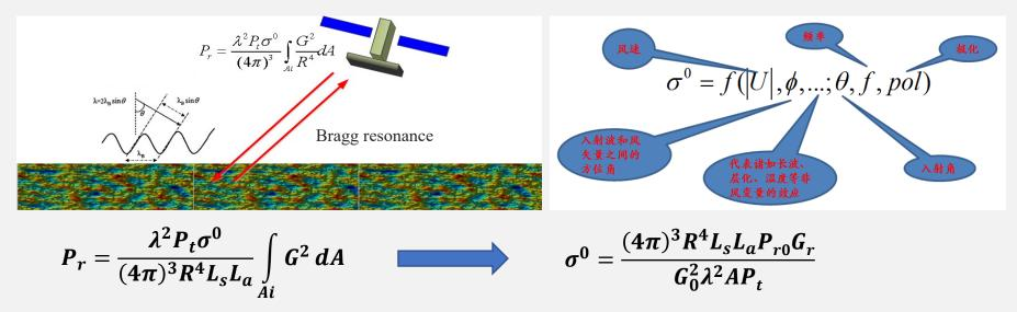
The ocean surface vector winds can be inferred from the measured Normalized Radar Cross Section (NRCS) signal strength ( $\sigma^0$ ) by using the Geophysical Model (CMOD) Function (GMF).
