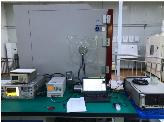
Prelaunch thermal cycling experiment
