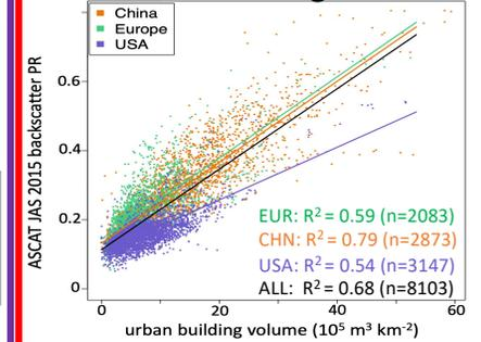
Mean summer 2015 ASCAT backscatter power return (PR) vs. building volume for urban grid cells (0.05° lat/lon) in 209 large cities in China, Europe, and the USA (building volume data from Li et al., (2020). Regional linear fits are shown as colored lines, linear fit for all data as a black line.
