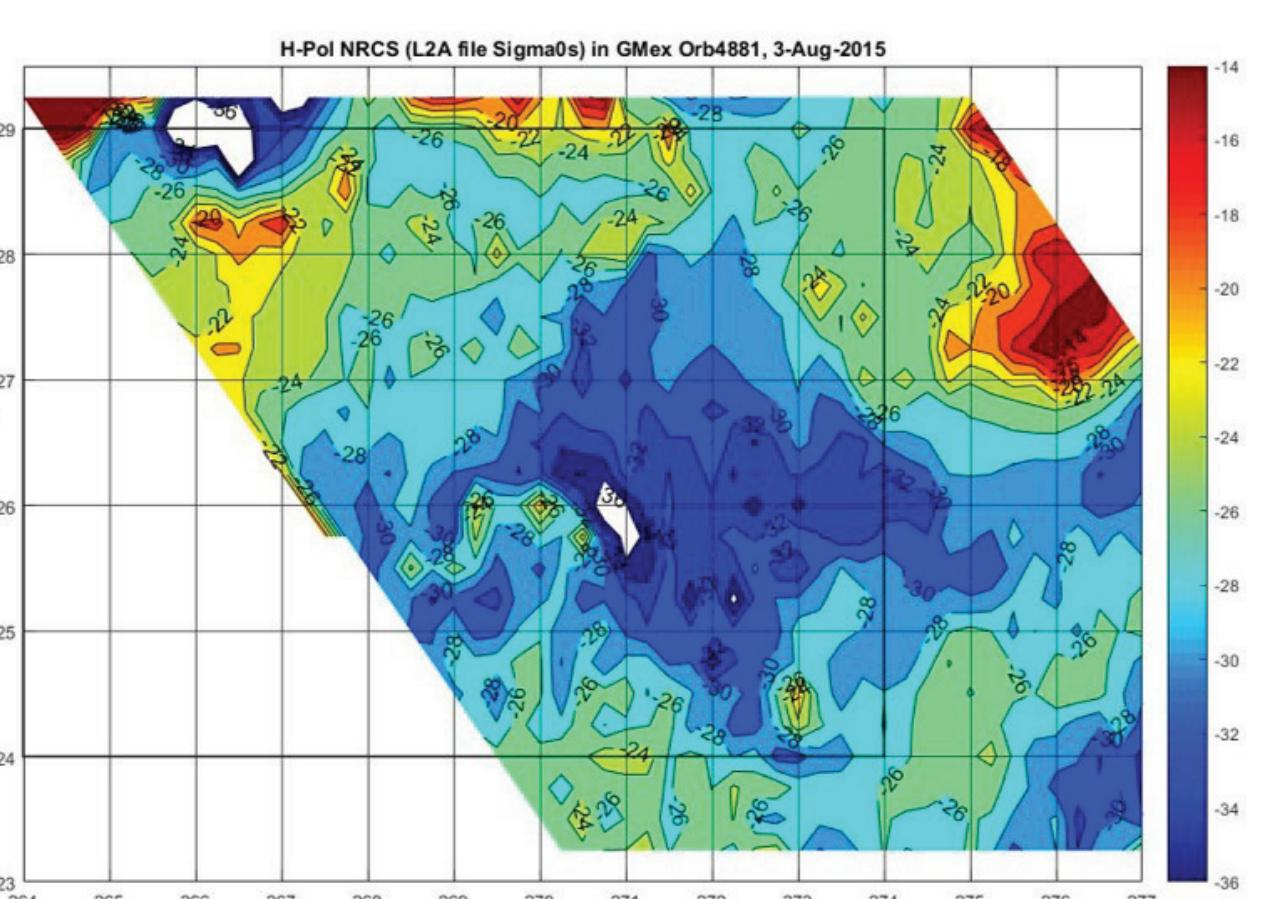
Figure 6. The RScat H-pol NRCS across region of interest. This is magnitude only, no look direction separation. The rectangle defined by the solid black line indicates a rain free zone that matches the wind map of Figure 2.
