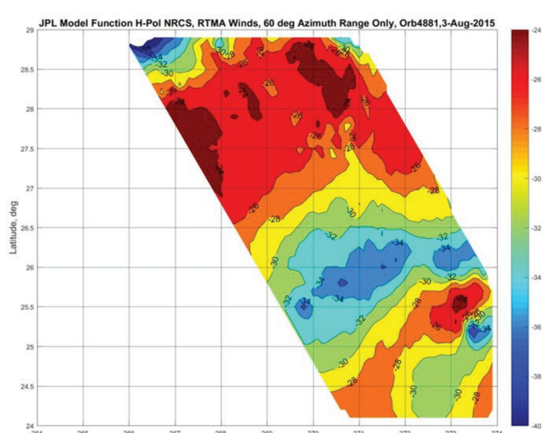
Figure 13. Estimates of the H-pol NRCS derived from the collocated wind vectors in Figure 3 and calculated using the JPL Model function at the locations where RScat measurements were made using on a 60° azimuth window.
