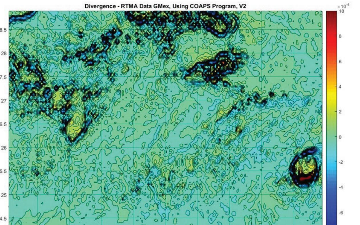
Figure 5a. Divergence of RTMA wind vectors shown in Figure 3.
