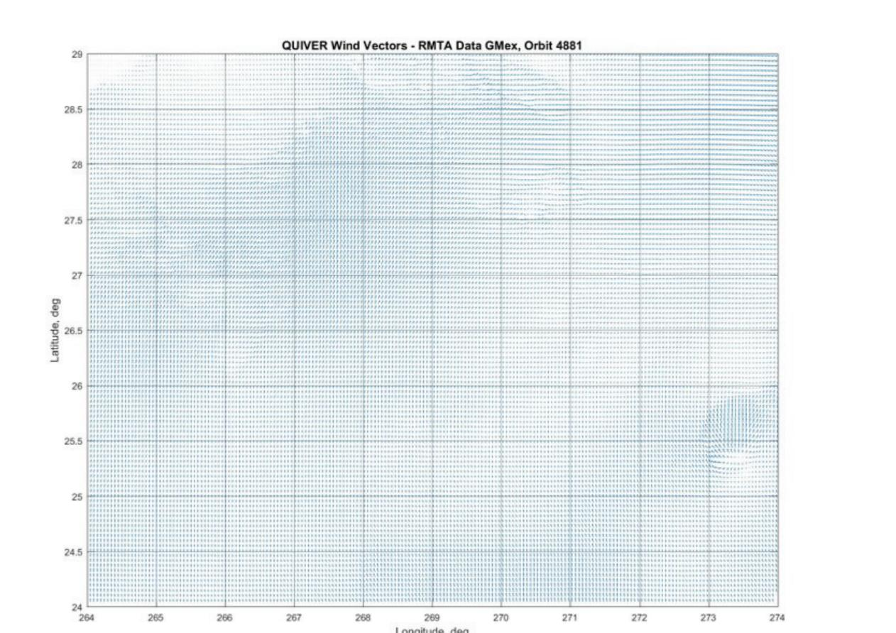
Figure 3. Wind speed vectors (magnitude and directions) associated with RTMA winds in Figure 2. The length of the arrows are scaled to represent wind magnitudes. Figures 2 and 3 indicate a wide range of conditions, including several areas with rapid changes in wind speed and direction, that will display distinct features of vorticity and divergence.
