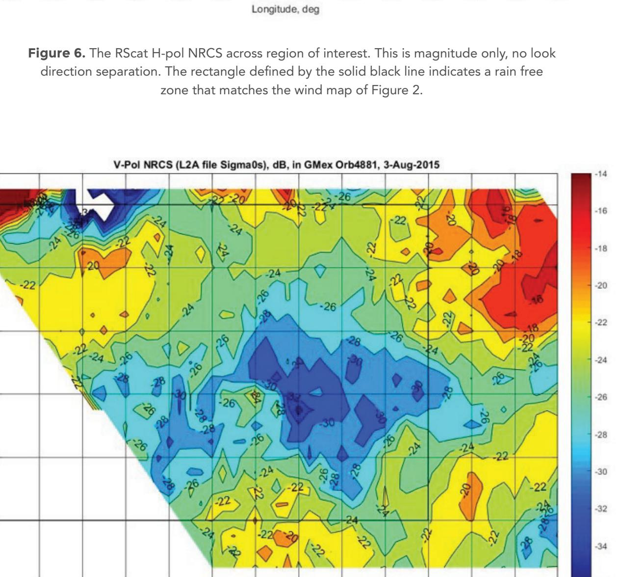
Figure 7. The RScat V-pol NRCS across region of interest. The rectangle defined by the solid black line indicates a rain free zone that matches the wind map of Figure 2.
