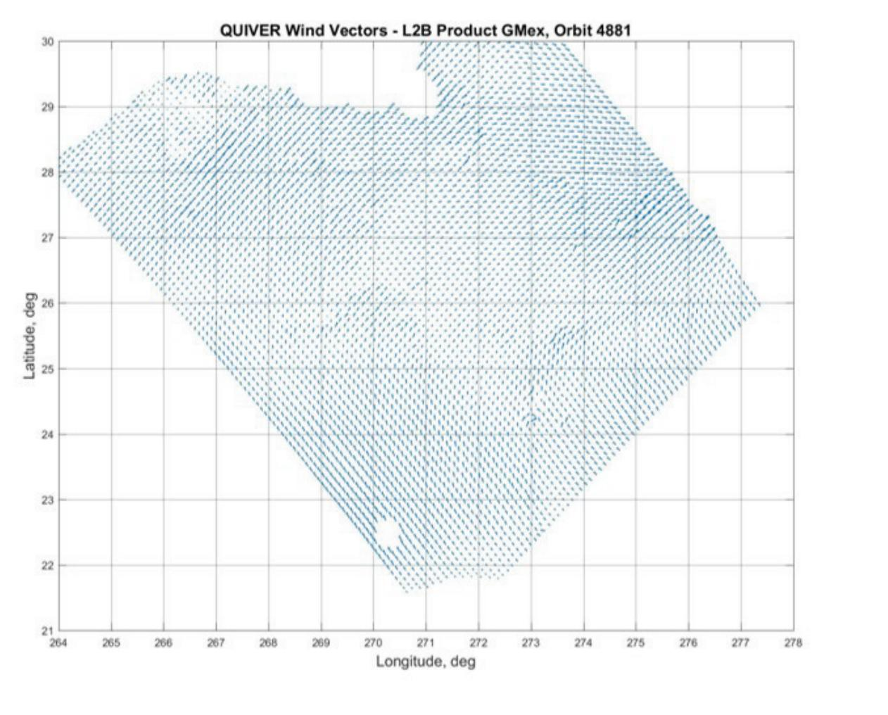
Figure 8. Map of the wind vectors for the JPL Level 2B Product. Correlations can be seen when comparing these results to the intensities and features seen in Figures 6 and 7.
