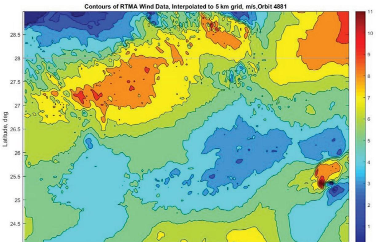
Figure 2. RTMA Wind magnitude,  $m/s$ , across region of interest, 5 km resolution. This is an hourly product that is based on an accumulation of multiple surface and space sensors. This image is within 25 minutes of RapidScat orbit 4881. The horizontal line at Latitude=28° demarcates a region to the north which is likely to be affected by rain.
