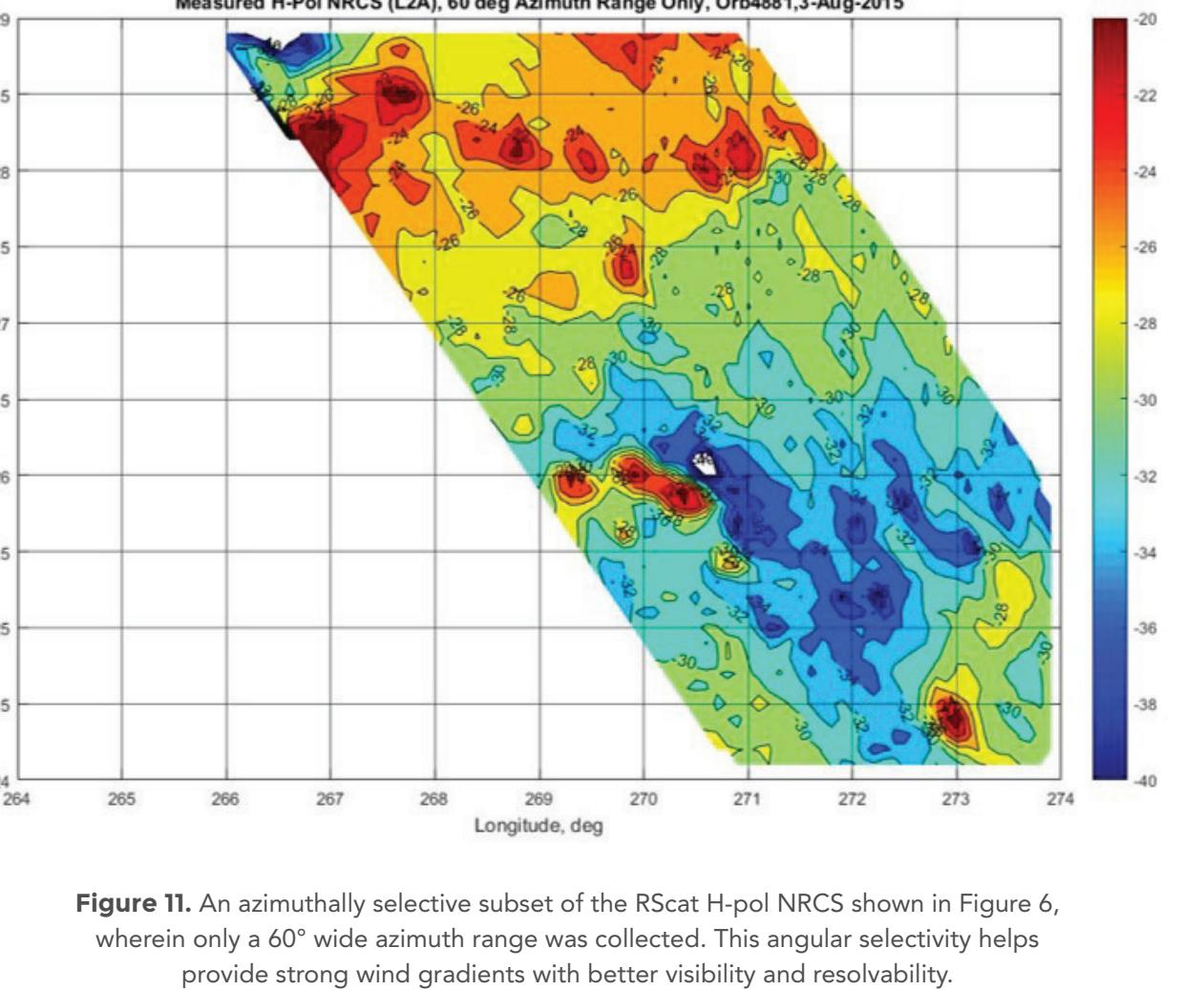
Figure 11. An azimuthally selective subset of the RScat H-pol NRCS shown in Figure 6, wherein only a 60° wide azimuth range was collected. This angular selectivity helps provide strong wind gradients with better visibility and resolvability.
