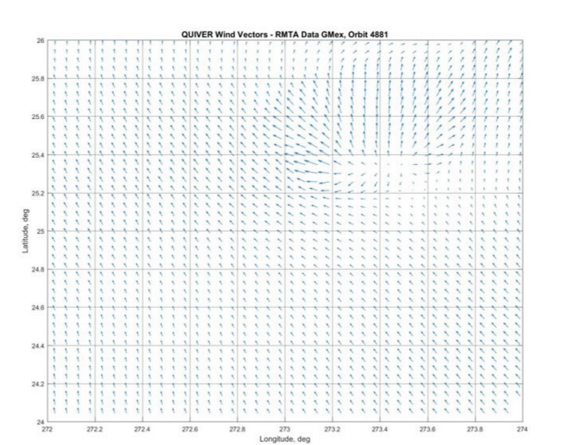
Figure 14. A subset ("zoom") area from Figure 3 that matches a feature in the model derived H-pol NRCS image in Figure 13, which displays strong variations in magnitude and direction.
