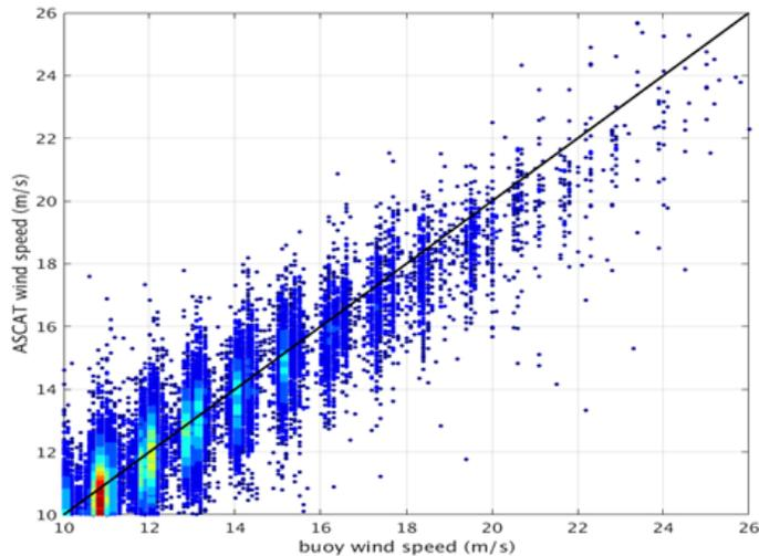
12.5 km ASCAT QC-accepted wind speed versus buoy wind speed
