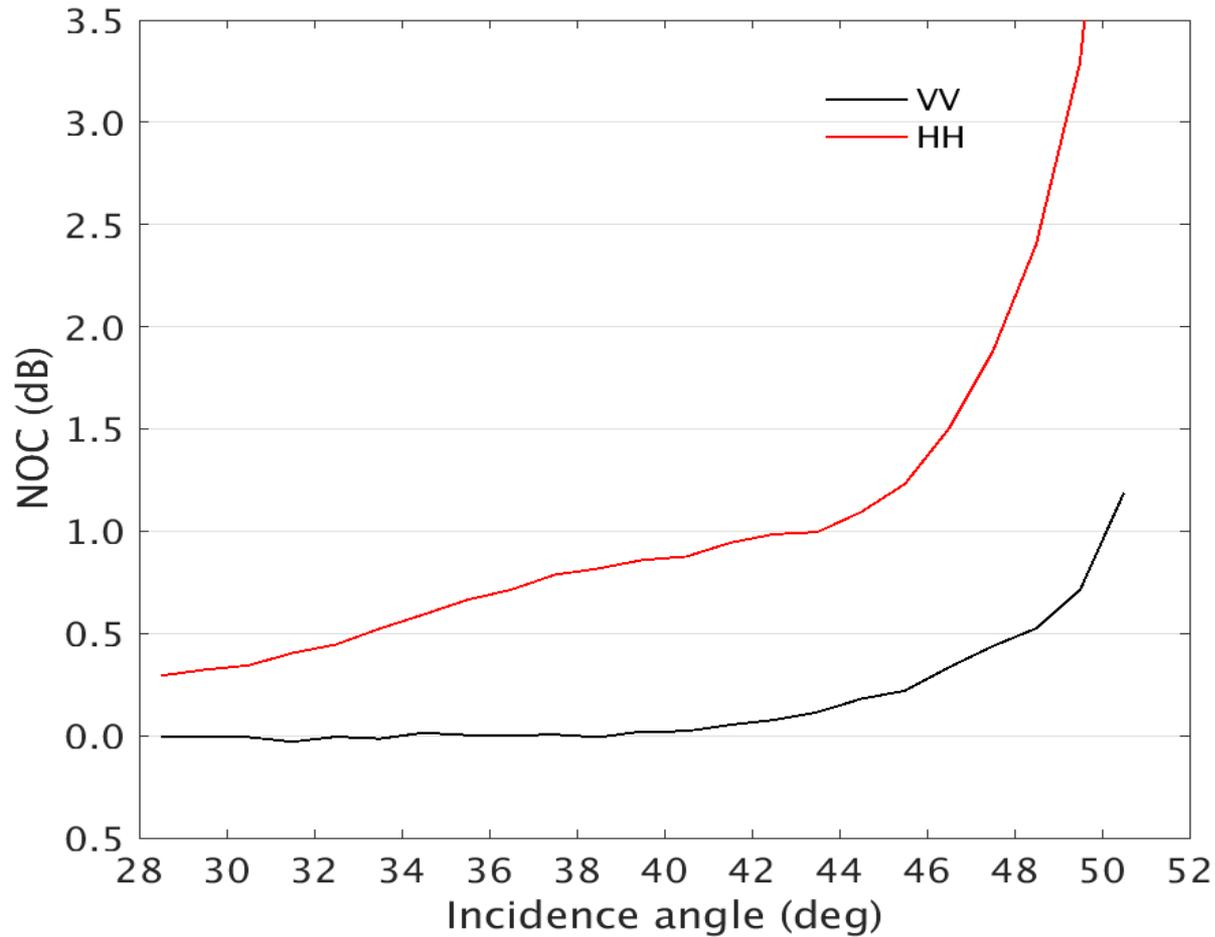
CFOSCAT NOC coefficients based on the **L2A** products
