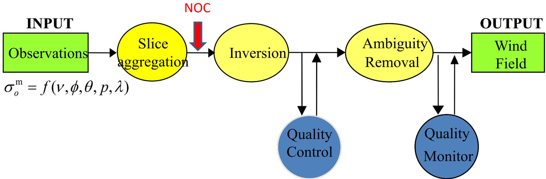
Similar to the conventional scatterometer wind retrieval, the L2 processing of CFOSAT scatterometer includes 1) slice aggregation, 2) wind inversion, 3) ambiguity removal, and 4) quality control.
