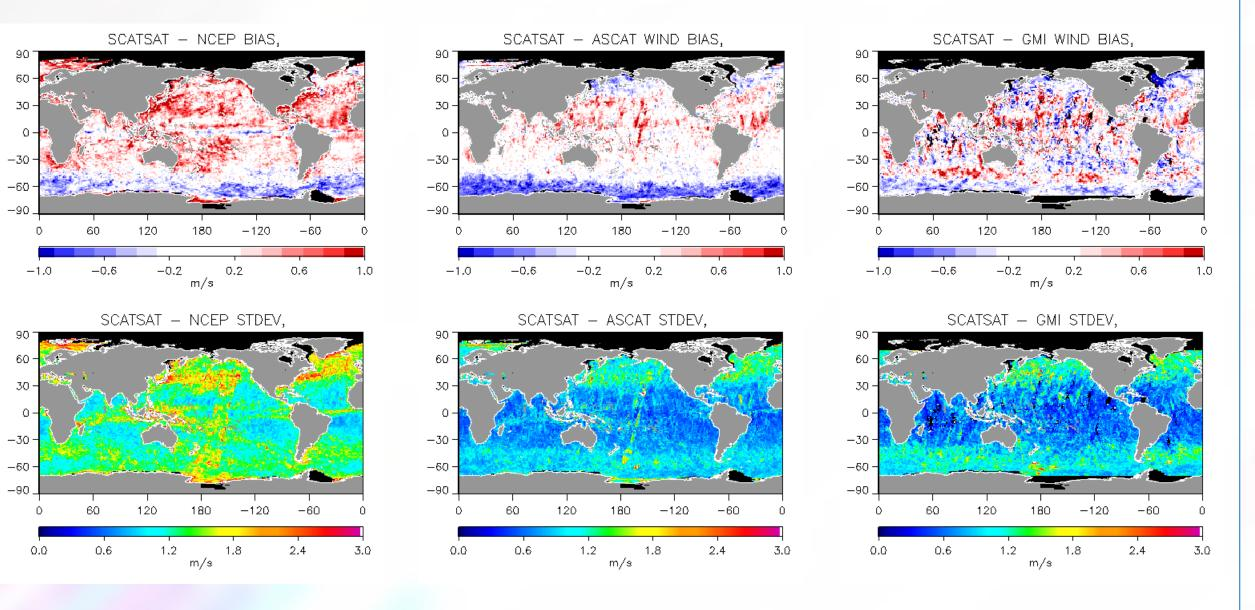
Shown above are global maps of ScatSat wind speed bias and standard deviation compared to NCEP, ASCAT, and GMI. In all cases, data displayed were rain-flagged in a very conservative way, using only ScatSat wind observations for which radiometers rain observations were available within 90 minutes. Overall, ScatSat winds display a negative bias in the Southern Ocean, likely due to the impact of cold SSTs on Ku-band radar backscatter. Another regional bias appears in the Northern midlatitudes.
