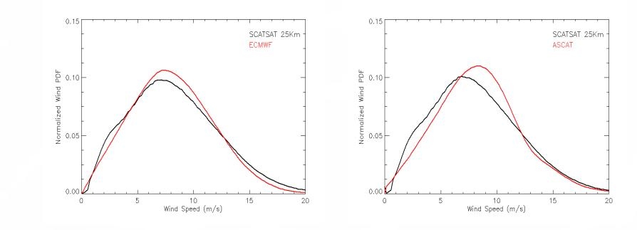
ScatSat 25 km wind speed PDFs are in reasonable agreement with ECMWF, and with ASCAT. The bump in the PDF for winds below 5 m/s is a common spurious feature for scatterometers' PDFs, and is likely due to a small discontinuity in the Geophysical Model Function for winds below and above this wind speed. It can be easily be fixed by imposing a smoother transition for the GMF coefficients.
