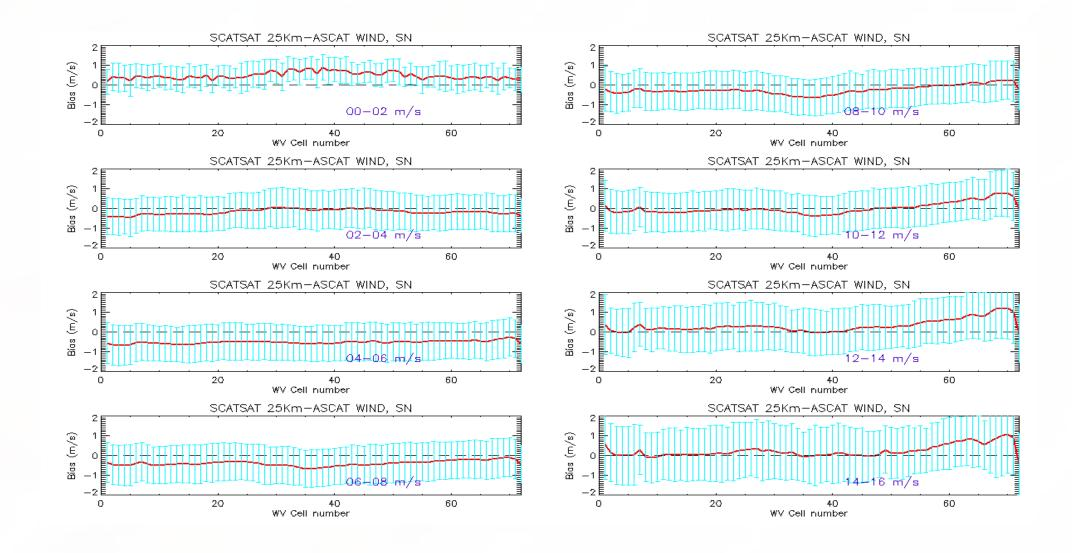
The figure above displays ScatSat wind speed bias compared to ASCAT as a function of the wind vector cell (WVC) position along the swath, and for different wind regimes. ScatSat wind speeds are remarkably free of across-track bias for 0-10 m/s wind speeds, for both descending (figure above) and ascending (not shown) passes. For winds greater than 10 m/s, a bias up to 1 m/s emerges on the left side of the swath for both asc/desc passes.
