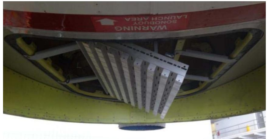
Aft-looking picture of the C-band antenna.
