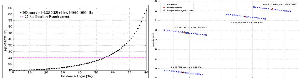
Figure 7 (left): plot of the sqrt of scattering area as a function of incidence angle, for the delay-Doppler window selected. The 25 km CYGNSS baseline requirement is also shown. (right): Graphical illustration of how time averaging works.
