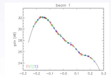
Set of transponder data with fitted gain model
