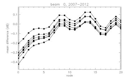
Oscillations in the difference between sea ice backscatter and ice line model in the left fore beam, 2007-2013
