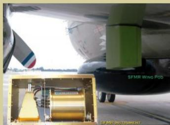
Figure 2: Picture of the SFMR wing pod installed on the aircraft and the SFMR instrument itself. (image source: www.prosensing.com)
