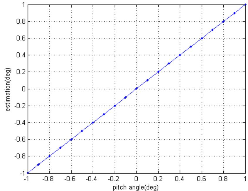
The STD of **pitch** angle estimation is  $<0.001\text{deg}$
