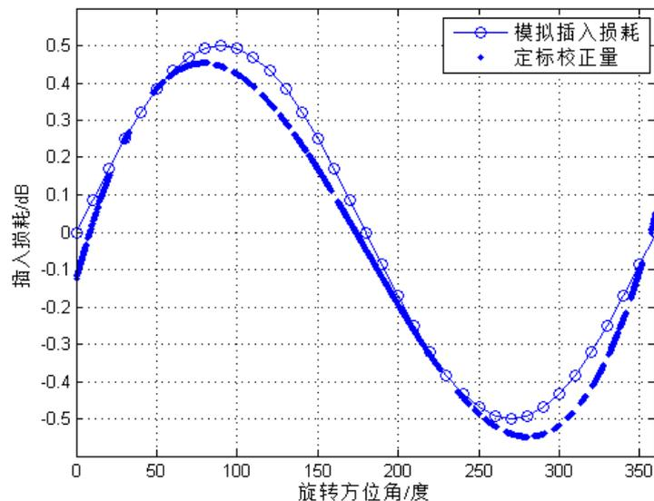
The estimation result of the loss due to rotary joint (STD  $< 0.05$  dB)
