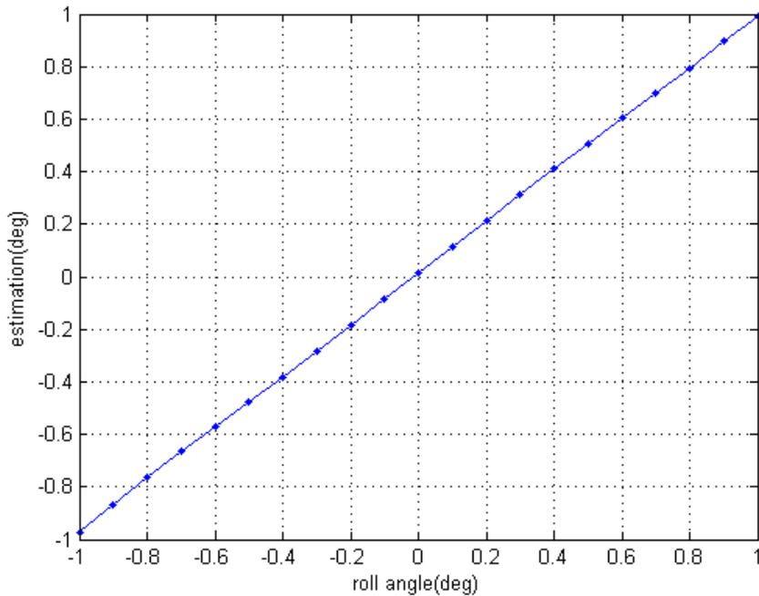
The STD of **roll** angle estimation is  $<0.02\text{deg}$
