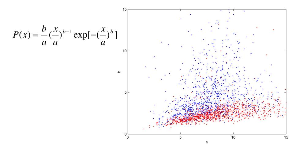
The relation between a and b of Weibull distributions from AMSR-E (blue) and CALIPSO (red).
