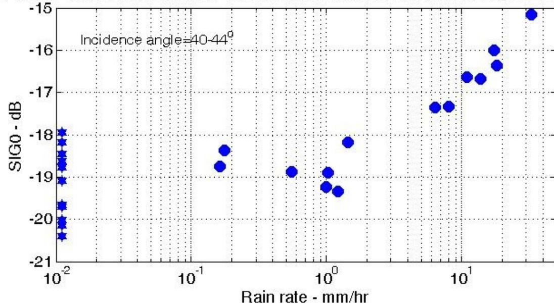
ASCAT - NRCS vs Rain Rate, Aft Beam, Sequence of Incidence Angles, 19-Apr-09
