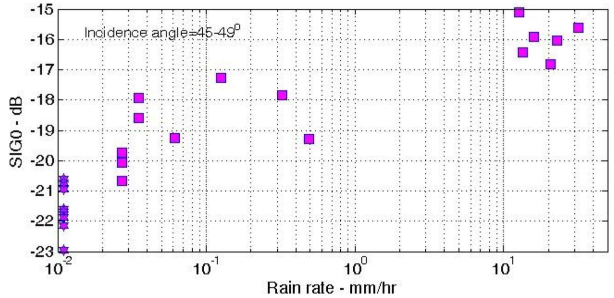
ASCAT - NRCS vs Rain Rate, Mid Beam, Sequence of Incidence Angles, 19-Apr-09
