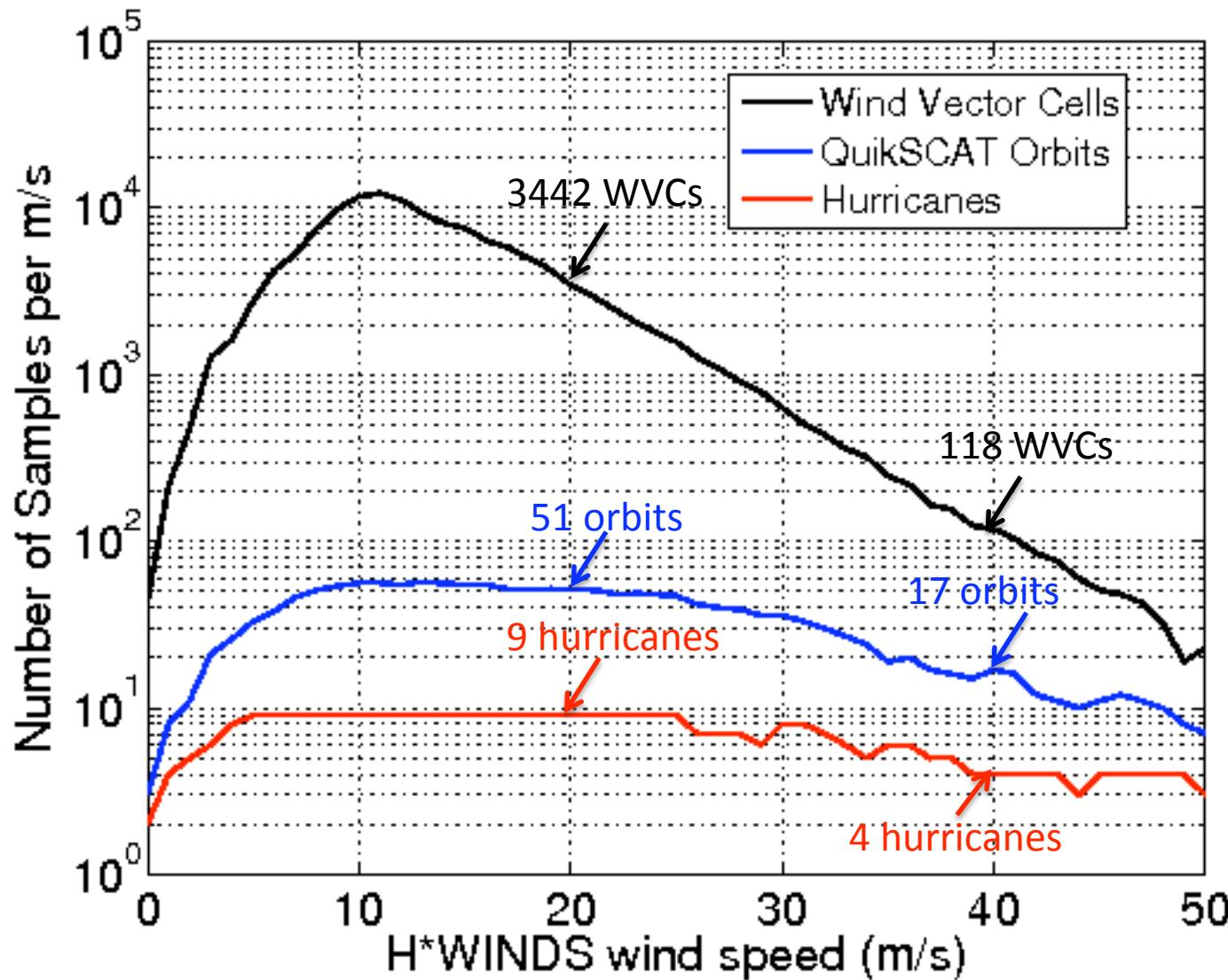
Because of the rapid decline in samples with speeds, we weighted high wind samples more heavily during network training.
