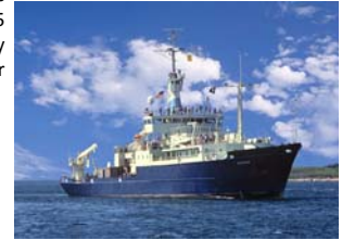
Figure 2. Research vessel Knorr with meteorological instrumentation on a bow mast.
