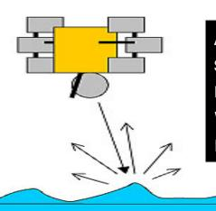
A radar signal is sent to the surface. It bounces off short waves (2-6cm). The microwave energy received back at the satellite is the signal  $\sigma_o$ . Thus we get a measure of the small-scale roughness. Sailors know this is  $\alpha$  windspeed
