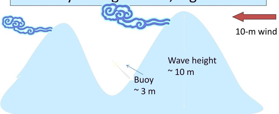
Sheltering: The high waves place the buoy in shelter and/or turbulent wake of the waves yielding low winds
