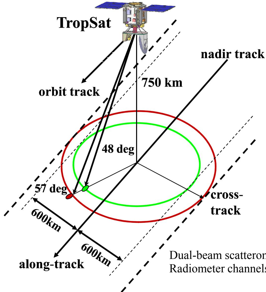
Dual-beam scatterometer channels
